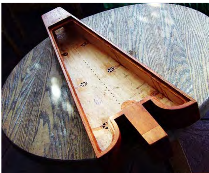
Inside view of the finished soundbox of the Downhill Harp reproduction, showing how the top of the box is hollowed right through. (Photograph ©2009 by Michael Billinge, used by permission.)
