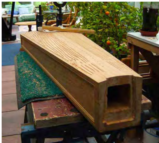
Using an improvised "scratch-stock" to cut grooves as a depth guide prior to finishing the face of the soundbox. (Photograph ©2009 by Michael Billinge, used by permission.)
